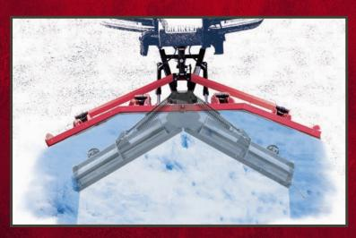
The Hiniker Scoop's concave shape captures more snow than other plow designs. Its concave design and fixed-end simplicity provides operators an effective and efficient plow for a wide range of applications.
