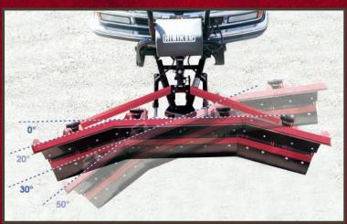
The ability of the Hiniker Scoop plow to angle full right or full left for conventional plowing, combined with the outer end's 50-degree forward angle, significantly reduces high-side spillage. The Scoop plow is ideal for parking areas and large lots where high-capacity, high-efficiency plowing is essential.
