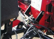
One pass plowing . . . no problem! **Hiniker's pitch adjustment** levels the blade to assure full ground contact for optimum cleaning efficiency.
